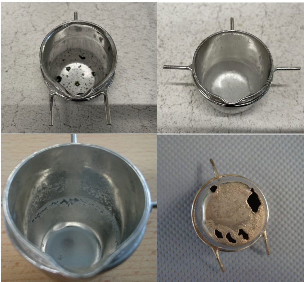
Figure 1: different types of damage to the crucible
