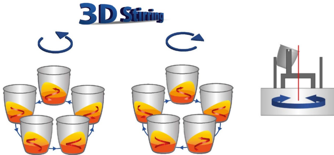
Figure 4: Application of the rotation stirring principle in the crucibles with the VITRIOX® ELECTRIC
