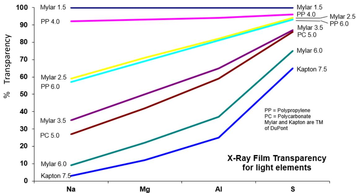
**Polypropylene** is especially suited to the trace analysis of solid samples, as it has no major contamination in it. In contrast, **Mylar** contains the undesirable phosphorus and calcium (3.5 µm Mylar corresponds to 50 ppm Ca and 250 ppm P in a straight oil, e.g., clean white oil).
